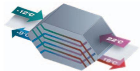
Plate counter-flow heat exchanger
