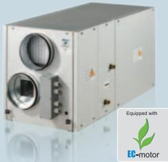
Air handling units with air capacity up to 550 m<sup>3</sup>/h and recuperation efficiency up to 95% in sound- and heat-insulated casing with water heating coils.
