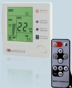
Used for temperature mode control in ventilation, heating and air conditioning systems. This temperature regulator can be used for control of the fan and fancoil dampers, the air heating units with 230V three speed fans and operates as an automatic heating or cooling controller.
