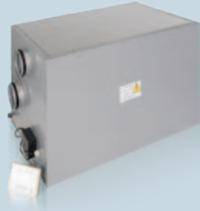
Air handling units with the air capacity up to 2200 m<sup>3</sup>/h and recuperation efficiency up to 85% in sound-proof and heat-insulated casing with electric heater.
