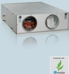
Compact suspended air handling units with air capacity up to 3800 m<sup>3</sup>/h and recuperation efficiency up to 90% in sound-proof and heat-insulated casing with electric heater.
