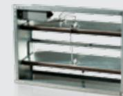
Smoke dampers installed on the protected premises accept smoke fumes and channel them into smoke shafts. Such devices are equipped with electromagnetic or electric actuators. The dampers are rated according to the fire-resistance limit which can vary up to 180 minutes at the smoke temperature of 600 °C.
