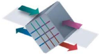
Principle of operation of plate heat recovery of cross-flow type
