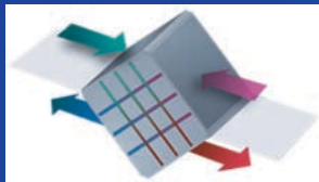
Cross-flow heat exchanger operating logic
