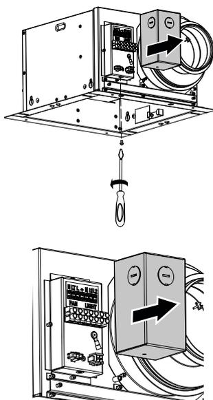
Remove the protective cap and install the cable gland.
