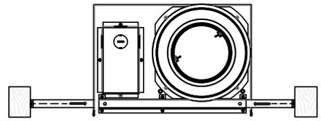
Additional fastening holes in the fan casing may be used for mounting purposes
