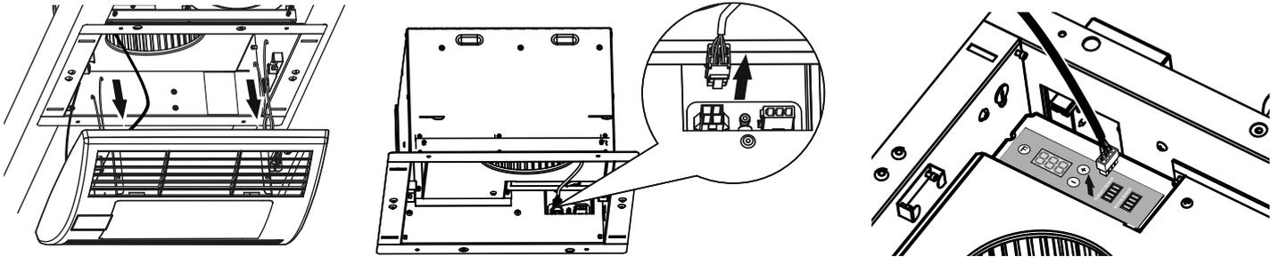
2. Take off the surface-mounted luminaire. Press the holders on the reverse side of the grille frame and take off the surface-mounted luminaire.
