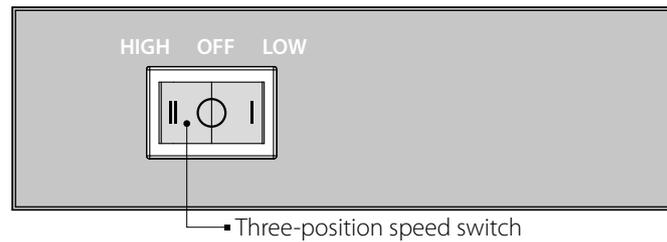
The fan with AC motor is controlled by a three-position switch. The switch has three positions:
