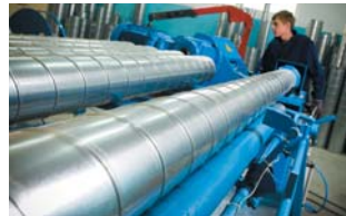
Spiral air ducts workshop
